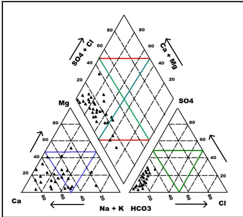
Figure 15: Piper diagram for representing ground water analysis
