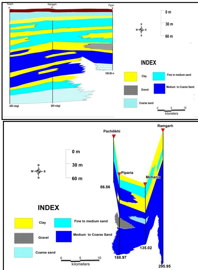
Fig: Aquifer disposition along Ramgarh block
