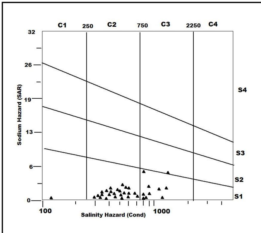
Figure 16: Wilcox diagram to represent relationship between salinity and sodium.
