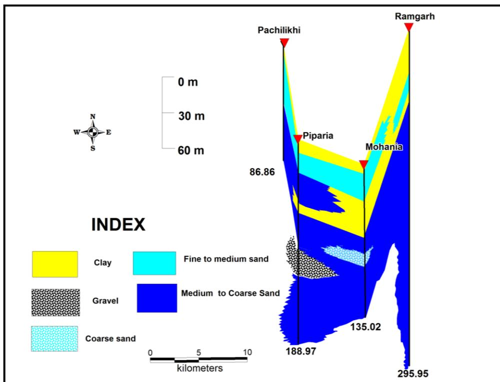
Figure 20: 2D Hydrogeological section from Pachilakhi to Rampur
