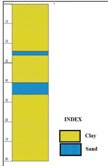
**Fig: Lihtological log of exploratory well at Chainpur block.**
