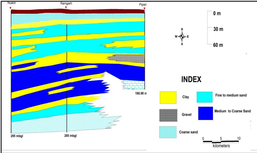
Fig: Aquifer disposition along Nuaon block
