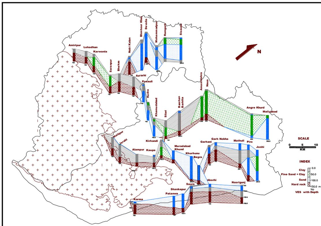
Figure 22: 2D Geophysical section along Kaimur to Rohtas district
