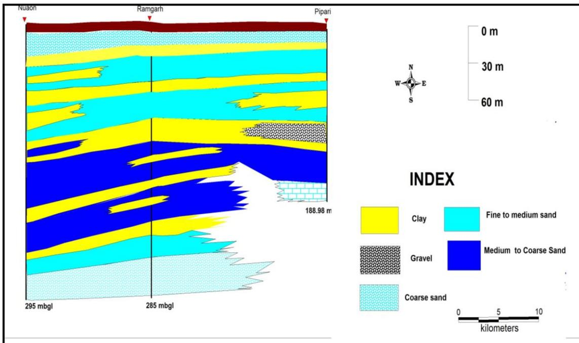
Figure 21: Hydrogeological section along north-south transect from Nuaon to Piparia
